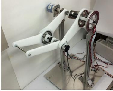
Fig. 3. Real robotic arm using rotational counterweights
