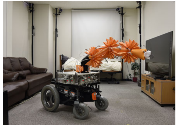
Fig. 1. Inflatable robotic arm on a mobile platform in living space
