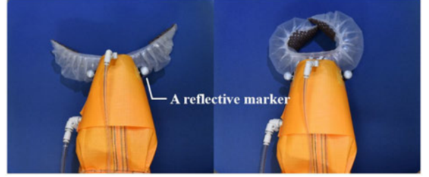
Fig. 4. Robotic gripper using a pleated sheet structure
