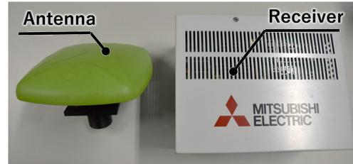
Fig. 3. Quasi-Zenith Satellite System module (AQLQC-V, Mitsubishi Electric Inc.)
