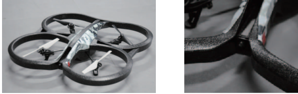
Fig. 5. Parrot Ardrone 2.0 and front camera
