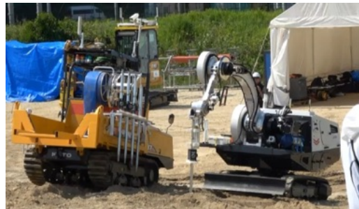
Fig. 5 Experiment of transporting and installing Pile-type Sensor Pod
