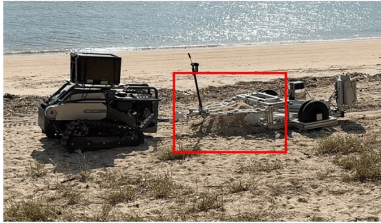
Fig. 14 System in a stopped state due to the deposited sand.
