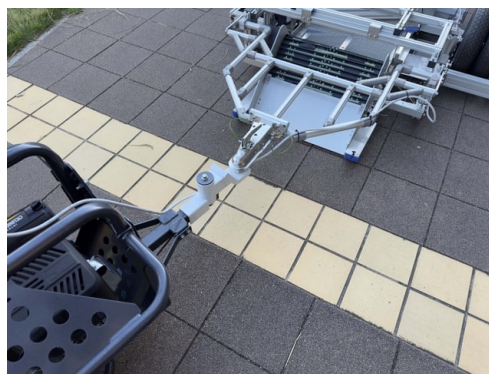
Fig. 9 The coupling structure of two robots.
