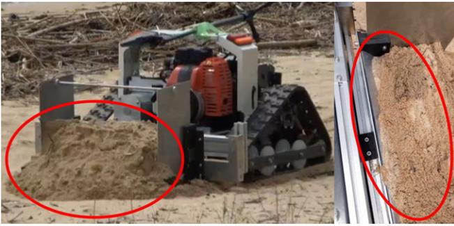
Fig.16 Excavation by 40° claw
