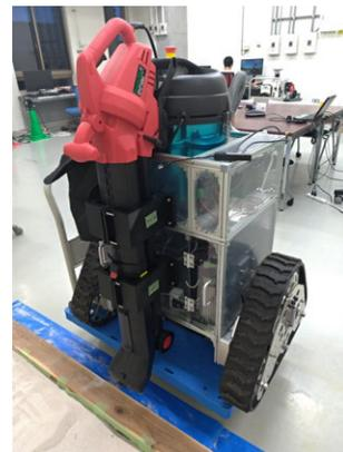
Fig.2 Vacuum-type marine microplastics cleaning robot<sup>[4]</sup>
