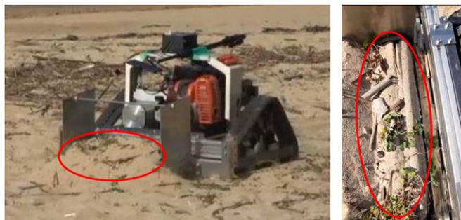
Fig.21 Excavation by claw with crawler
