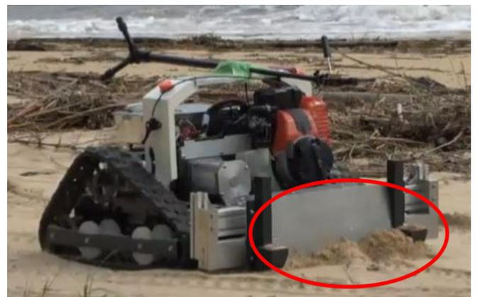
Fig.15 Excavation by 80° claw
