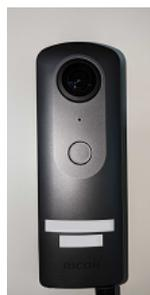
Fig. 5 360° camera (Theta V, RICOH)
