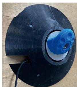
Fig. 1: Appearance of hold force measurement system[2]
