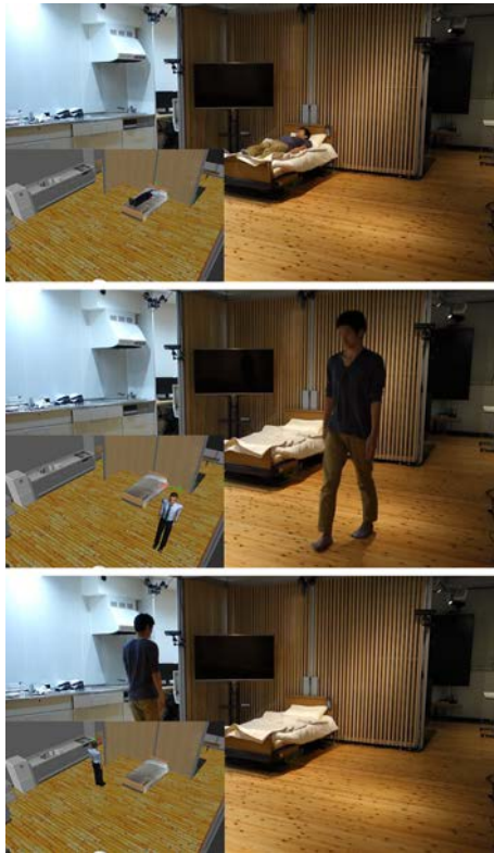
Fig. 4: Tracking of care receiver by UWB beacon
