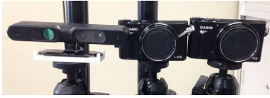
Fig.7 Measurement system composed of one RGB-D camera and two high speed cameras.
