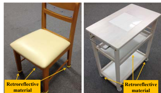
Fig. 4 Position of retroreflective material
