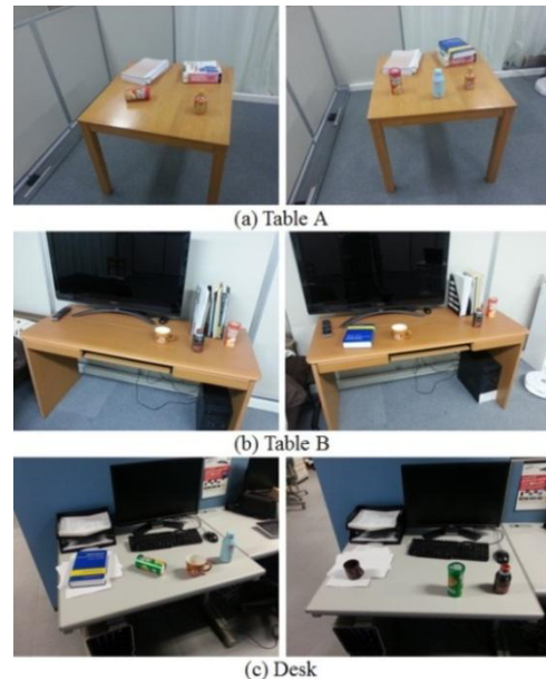
Fig. 4 Test data for change detection: (Left part) Memory data, (right part) Newly captured data. One set has two data which are captured in time and different point of view of a Kinect sensor.
