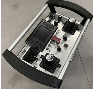
Fig.3 The embedded systems (Cat Command, Caterpillar Inc.) used in the proposed retrofit system.
