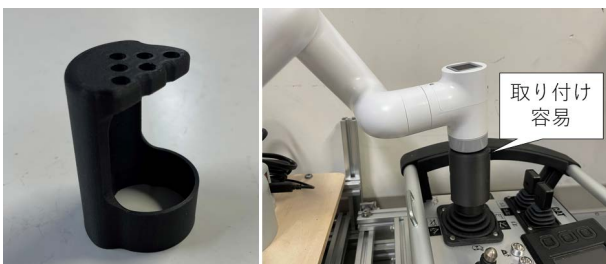
Fig.5 Mounting device used for retrofitting.
