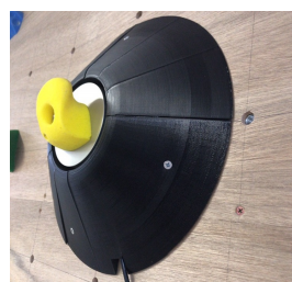
Fig. 1: Appearance of hold force measurement system[2]
