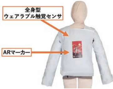
Fig.2 Attaching the tactile sensor to the doll
