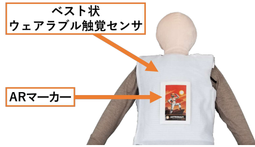
Fig.5 Attaching the tactile sensor to the doll
