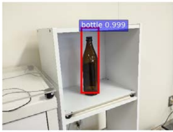
Fig.2 Example of detection. Faster R-CNN detected the bottle in the shelf with the score 0.999 in 0.089s
