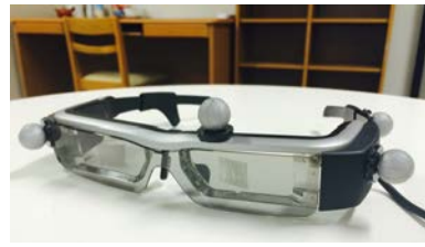
Fig.3 Smart glass (Moverio BT-200AV, EPSON) with markers
