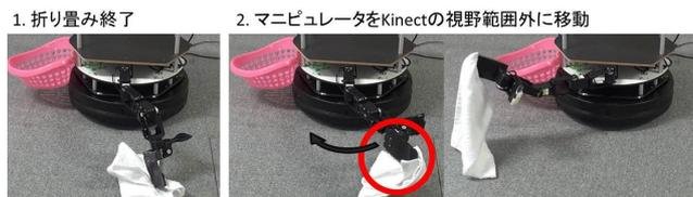
Fig.9 Failure of folding a towel
