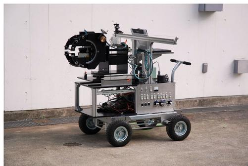
Fig.1 3-Dimensional Measurement Mobile
