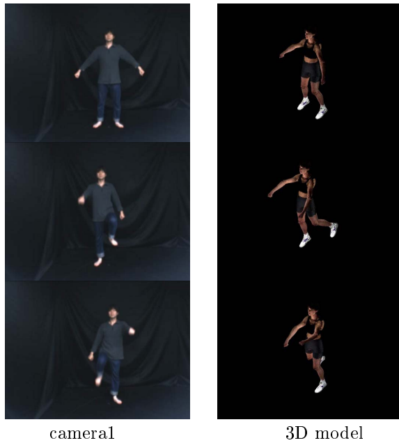
Fig.7: Tracking results by a single camera
