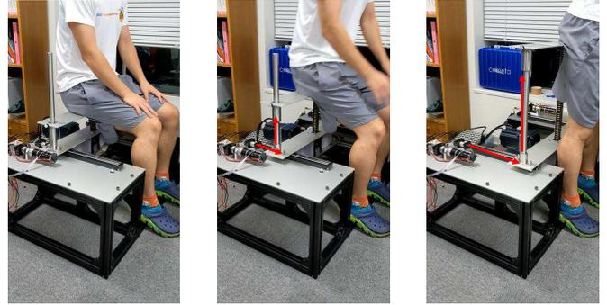
Fig. 4. STS motion with support by developed assistive device.
