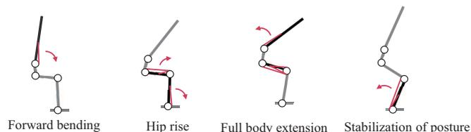
Fig. 1. The four phases of the standing movement
