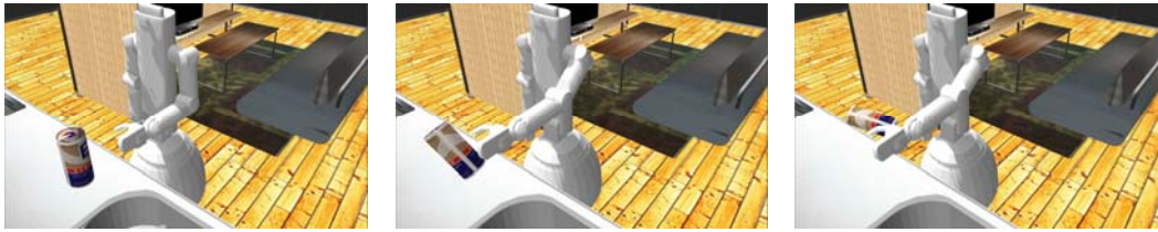
Fig. 3 Object grasping planned by dynamic simulator "Gazebo" and motion planner "MoveIt"
