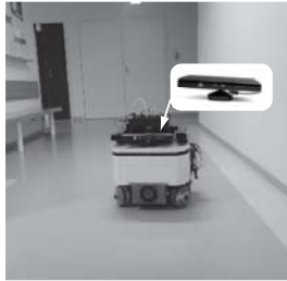
Fig. 6 Mobile robot equipped with RGB-D cameras (Kinect) [29]
