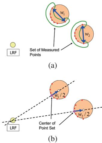
Fig. 8. Estimation of object position.
