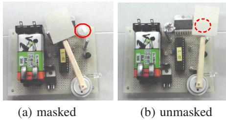
Fig. 11. Pyroelectric sensor unit with a chopper. A pyroelectric sensor is masked by a chopper in (a). The sensor is unmasked in (b).
