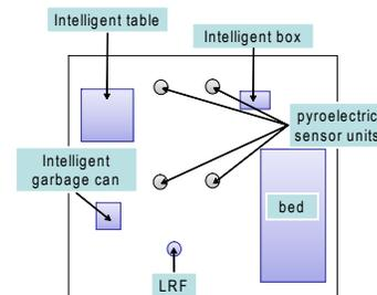
Fig. 13. Experimental setup.
