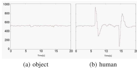
Fig. 12. Measurement result of a pyroelectric sensor unit with a chopper.
