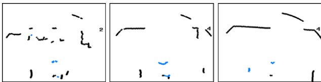
Fig. 7 (Color online) The images show examples of scans taken at the different layers. The left image corresponds to the lower layer (legs), the middle image to the middle layer (upper body), and the right image to the top layer (head). Blue points indicate segments classified as positive (body parts). Black points correspond to segments classified as negative (non-body parts)
