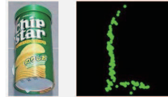
Fig. 4. A point cloud of an object measured by the sensed floor.
