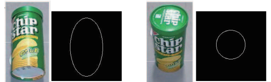
Fig. 8. The contour images of an object with different orientations.
