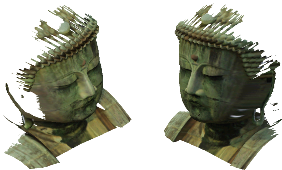
Figure 13: Aligned color texture on the 3D geometric model
