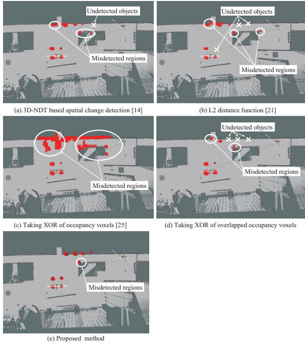
Fig. 5. Detected changes by (a) 3D-NDT based spatial change detection [14], (b) L_2 distance function [21], (c) taking XOR of occupancy voxels [25], (d) taking XOR of overlapped occupancy voxels, and (e) proposed method. Misdetection regions and undetected objects are indicated by white circles and crosses.
