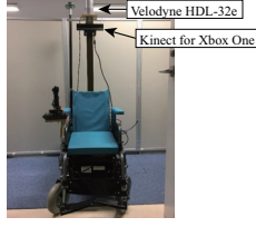
Fig. 1. Mobile robot system equipped with an omni-directional laser scanner (Velodyne HDL-32e) and an RGB-D camera (Kinect, Microsoft).
