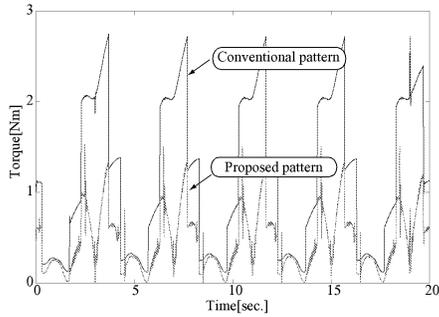
Fig. 16. Torque at knee joint of right leg (absolute value)
