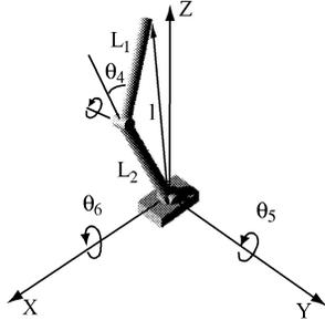
Fig. 7. Approximated calculation of Inverse Kinematics
