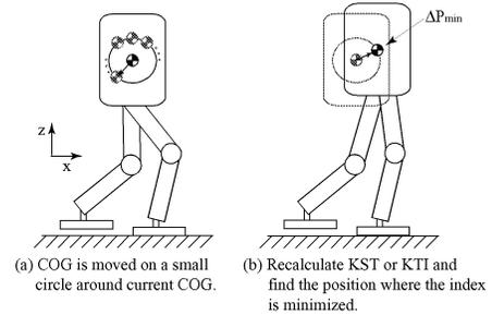
Fig. 6. Calculation of  $\Delta P_{min}$
