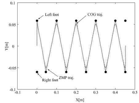
Fig. 3. An example of ZMP and COG trajectories projected on the ground for straight path
