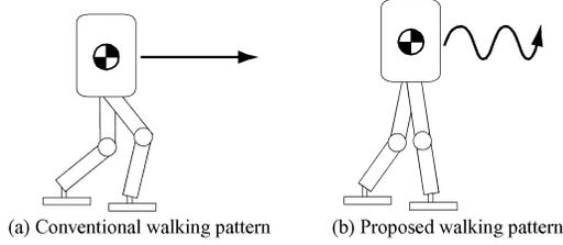
Fig. 2. Height control during walking
