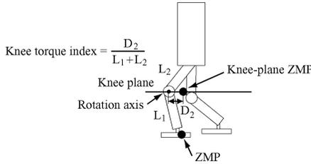
Fig. 5. Definition of Knee Torque Index
