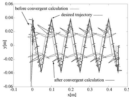
Fig. 12. ZMP trajectory before and after convergent calculation
