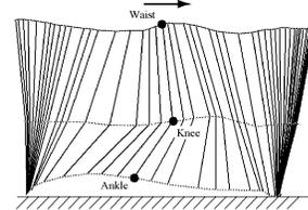
Fig. 1. Up-down motion of waist position while walking
