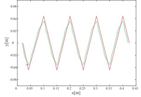
(b) ZMP trajectories using the original COG trajectory
