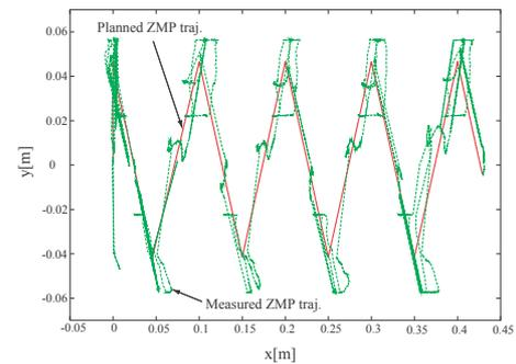
Figure 10: Measured ZMP trajectories
