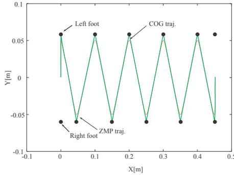
Figure 3: An example of ZMP and COG trajectories for straight path
