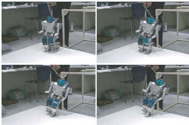
Figure 8: An example of walking experiments using HOAP-1 before convergent calculation (Walking speed 0.1m/s, Duty factor 0.75). The robot fell down just after starting walking motion.
