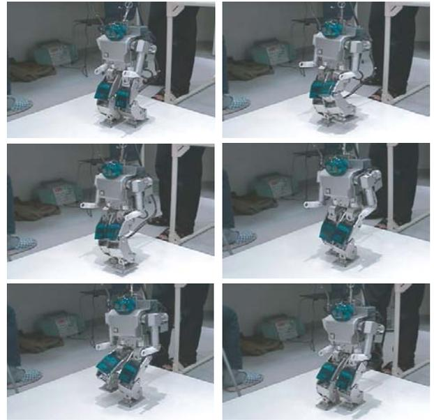
Figure 9: An example of walking experiments using HOAP-1 after convergent calculation (Walking speed 0.1m/s, Duty factor 0.75)
