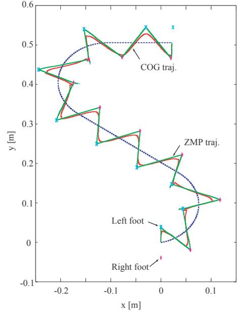
Figure 4: An example of ZMP and COG trajectories for curved path
