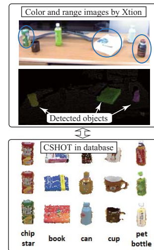
Fig. 6. Object detection on a table using a RGB-D sensor (Xtion) and CSHOT descriptor.
