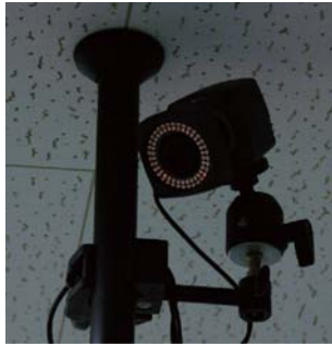
Fig. 10. Optical position tracking system (Bonita, Vicon)
