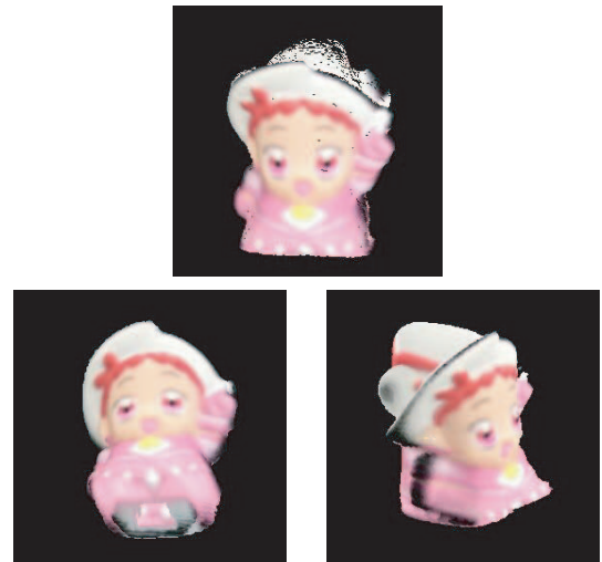
Figure 10. An example of mapping the camera image on the 3D model.
