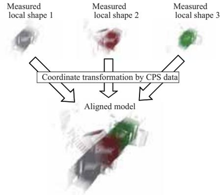
Fig. 6. Coordinate transformation by CPS information for creating aligned three-dimensional model
