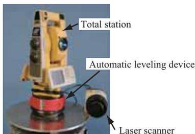
Fig. 7. Automatic leveling device
