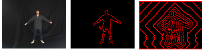
original image contour image 2D-Distance-Field Fig.3 Construction of 2D-Distance-Field
