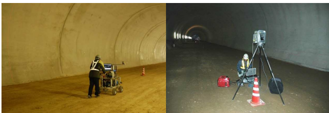
Fig.5 Measuring situation of 3DMMunit (left) & 3Dscanner (right)
