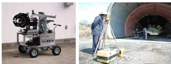
Fig.1 3-dimensional measurement mobile unit (left) and Situation of experiment that a simulated tunnel was used for (right)
