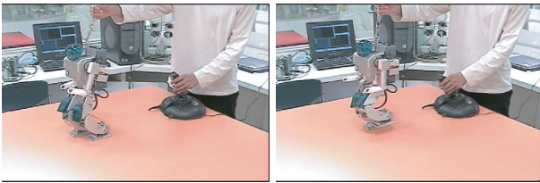
図 5: On-line walking pattern generation by joystick
