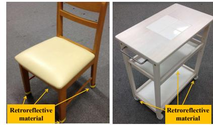
Fig. 8. Position of retroreflective material
