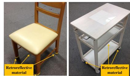
Fig. 8. Position of retroreflective material
