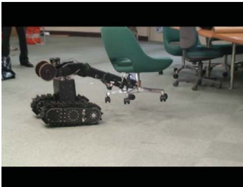
Fig. 2. HELIOS IX lifting a 7kg chair
