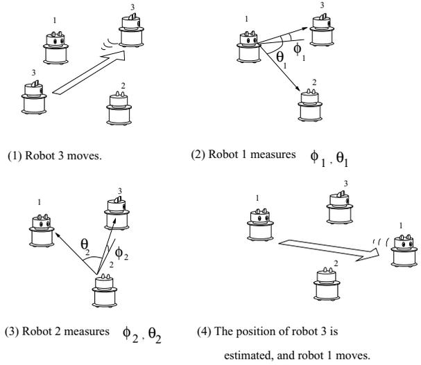
Figure 4: Cooperative positioning with multiple robots (Type II).
