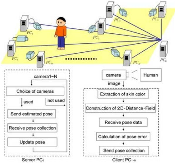
Fig. 5. Motion tracking using the distributed network camera system
