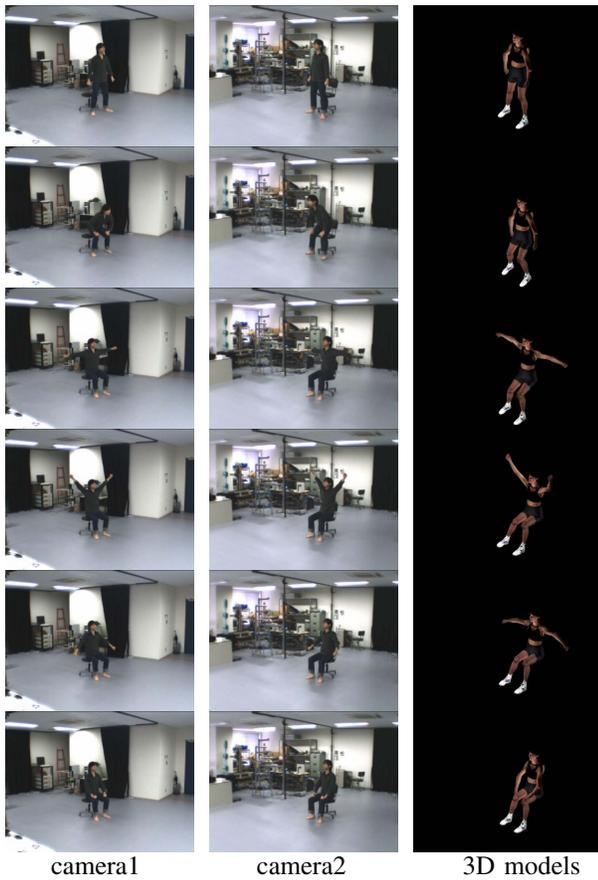
Fig. 7. Tracking results for sitting motion by two cameras
