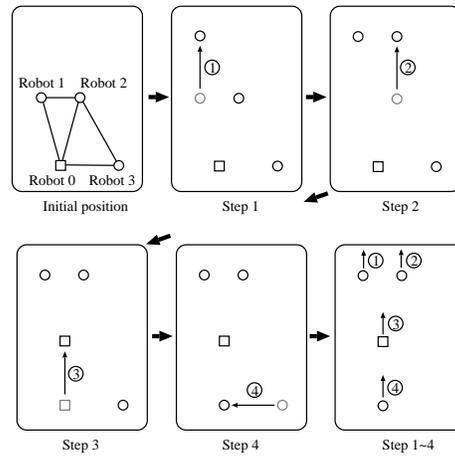
Fig. 11. Moving strategy in each measurement cycle.
