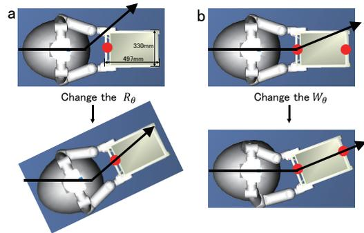
Fig. 8. Wagon path planning: (a) robot posture plan, (b) wagon posture plan.
