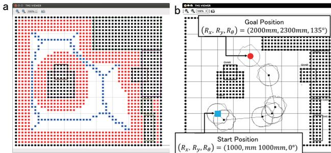
Fig. 6. Voronoi map and movement path: (a) collision area (red) and basic path (blue). (b) robot movement path.
