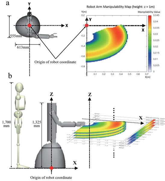
Fig. 3. Manipulability map for the robot: (a) 2D manipulability map for robot, (b) 3D manipulability map for robot.
