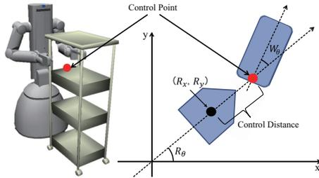
Fig. 7. Model of the robot pushing the wagon
