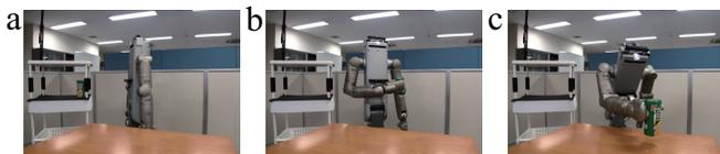
Fig. 11. Object gripping experiment: (a) initial state, (b) intermediate position, (c) object delivery attitude.
