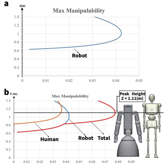
Fig. 4. Maximum value of manipulability: (a) maximum value of robot manipulability, (b) merge results for manipulability.
