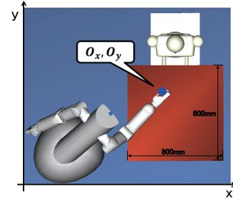
Fig. 12. Condition under which the object delivery experiment was conducted
