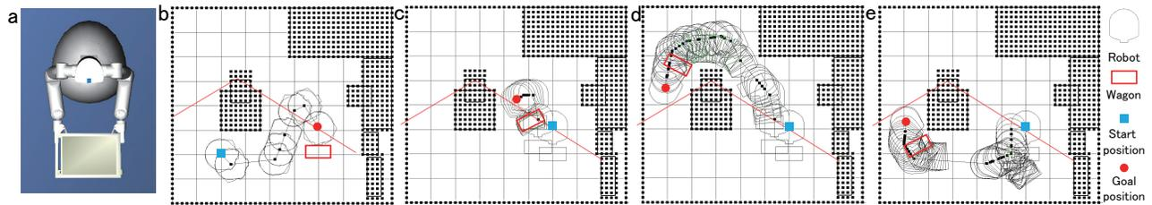
Fig. 15. Planning results for object delivery wagon route for holding candidate position using plan 1 : (a) holding candidate attitude, (b) robot path to wagon grip candidate 1, wagon route to object delivery position candidate 1,2,3 (c,d,e)
