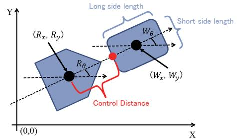
Fig. 1. Base position of the robot at the time of gripping the wagon ( $i = 2$ )
