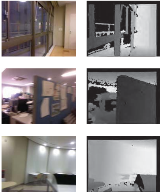
Fig. 5 Examples of misclassified pairs of RGB and depth images in experiment 1. In the upper row a scene of “kitchen 3” is categorized as a corridor. The middle row show an scene of “laboratory 4” categorized as an office. The bottom row shows a scene in “study room 2” categorized as a kitchen.
