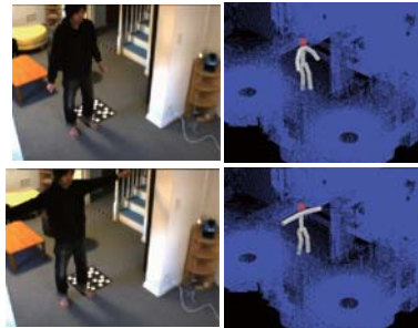
Fig. 8 Posture estimation of humans using captured camera images
