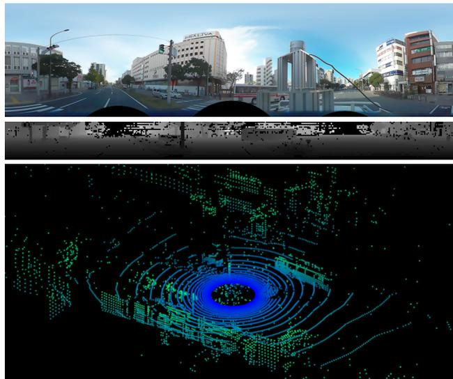
Fig. 1. Samples from the Sparse MPO dataset [13]. **Top**: Panoramic color image of the urban scene. **Middle**: Corresponding panoramic depth image directly obtained by LiDAR scanning. **Bottom**: 3D point cloud converted from the image. Panoramic depth image represents the surrounding geometrical information compactly.
