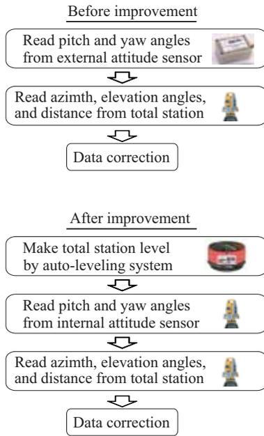
Fig. 9. Flowchart of data collection measured by total station
