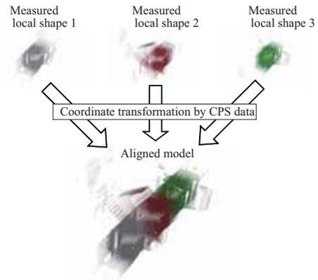
Fig. 6. Coordinate transformation by CPS information for creating aligned three-dimensional model
