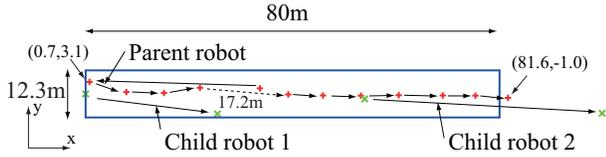
Fig. 19. Travel paths of the robots [m]
