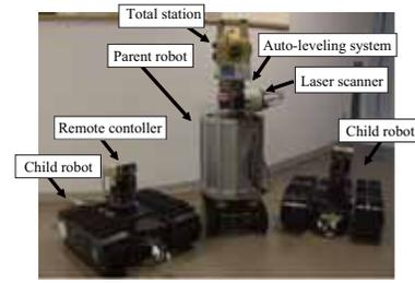
Fig. 2. The developed tunnel shape measurement system
