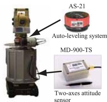
Fig. 8. Two-axes attitude sensor (MD-900-TS) and auto-leveling system (AS-21)
