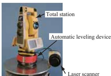
Fig. 7. Automatic leveling device
