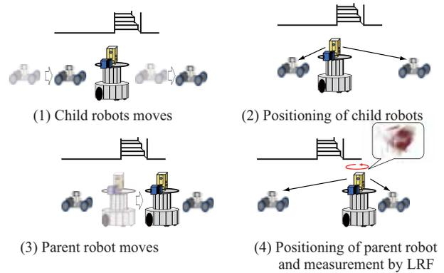
Fig. 5. Three-dimensional measurement using CPS and laser scanner
