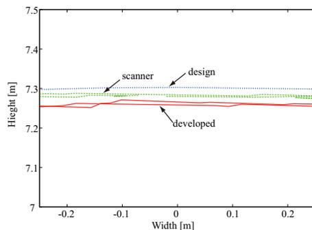
Fig. 25. Close-up of cross-sectional shape at 50m position
