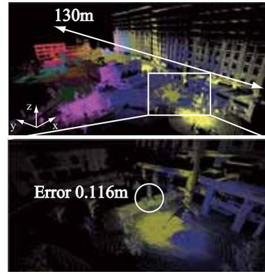
Fig. 15. Measured shapes and errors in outdoor environment
