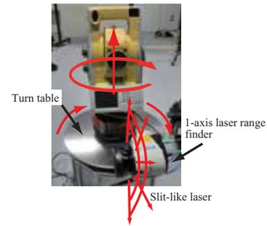
Fig. 3. Scanning system by 1-axis laser scanner and turn table
