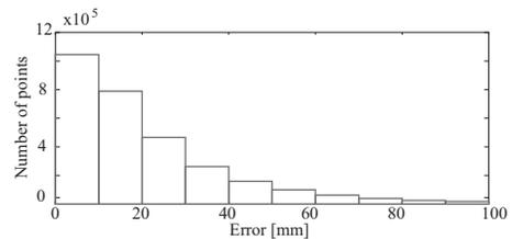
Fig. 23. Error histogram between the proposed system and the conventional laser scanner (TOPCON, GLS-1000)
