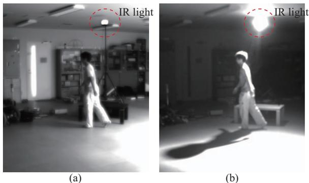
Figure 1. Examples of captured shadows projected by an infrared light, (a) the image with a visible light transmitting filter (this image is equivalent to how people see), (b) the image with an infrared transmitting filter.
