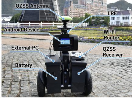
Fig. 13. Photograph of the tour guide robot
