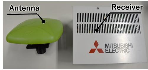
Fig. 3. Quasi-Zenith Satellite System module (AQLOC-V, Mitsubishi Electric Inc.)
