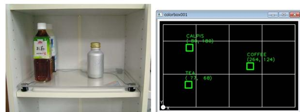
Fig. 6. Position measurement of objects.
