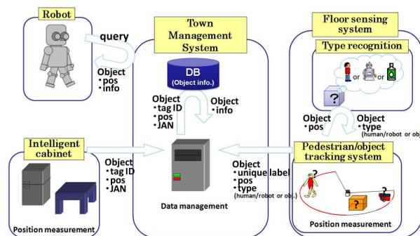
Fig. 2. Data flow of object tracking system.
